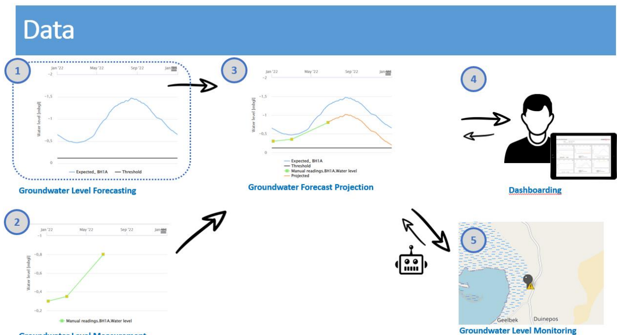
Figure 6. Data processing. 1) Forecasting groundwater level offline using a dedicated spreadsheet. 2) Direct collection of field measurements. 3) WaterMager projects the forecast based on latest measurements. 4) Data is accessible through dashboards. 5) System monitors potential violation of future groundwater level.
