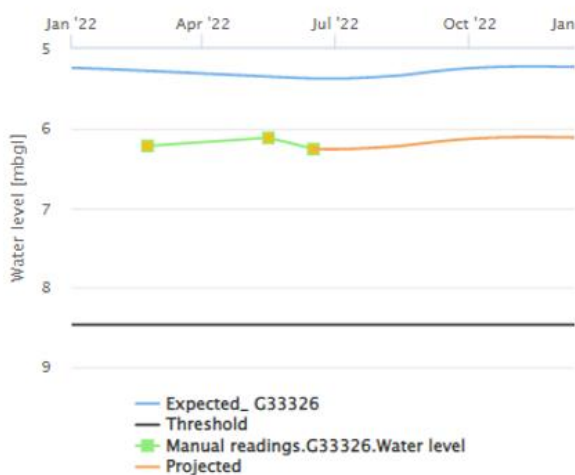
Figure 5. Expected seasonal variation in groundwater level at control point #1 (blue curve) together with monitoring data (yellow points), the design criteria (DC, orange line) and the projected groundwater head (green curve).
